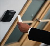
Access Control is quite simply how you control other people's access to your property. An access control point can be an external gate or door, or an internal door. Access is controlled through either a magnetic lock or electric strike and can be controlled using either a fob or keypad. It is a highly versatile means of protecting your property and can be used in conjunction with entryphones.
